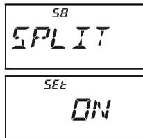
When the Split Tone feature is activated, you can see the following additional parameters following the “RV TN” parameter (while selecting the tone mode by pressing **[F/W]** → **[MODE(SP S)SQ TYP]**):
