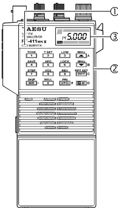
Remember to press the [F/M] key first (momentarily, unless otherwise indicated) when you want to use an alternate key function. All key functions are described in the “Operation” section, and summarized on the •*FT-411 MK Operator’s Quick Reference Card.*”
