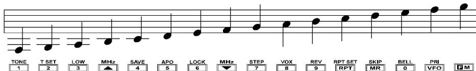
Feel free to use the keypad as a piano when the keypad is locked (who said we would couldn't fit a piano in a hand-held?). The only key combination that will affect transceiver operation is **[F/M]** followed by **[LOCK(6)]** within three seconds, which unlocks the keypad.
