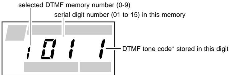
\*: DTMF codes are displayed as 0-9, A, b, C, d, E (for \*), F (for #) and “-” for empty (none stored).
