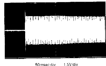
Figure 10: TS-870S attack characteristics
