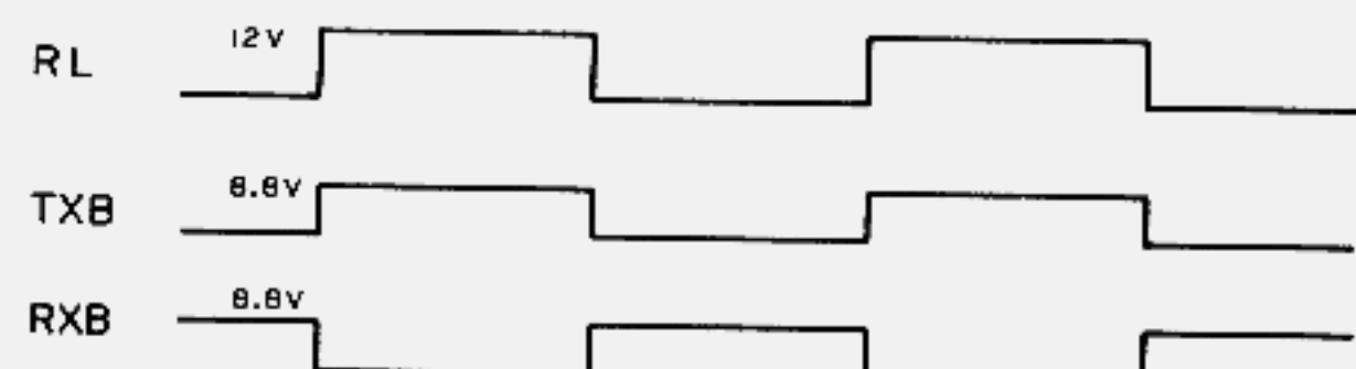
Fig. 10 STANDBY keying timing chart
