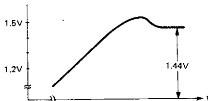
Fig. 6 The pin voltages while the Ni-CD Battery is charging
